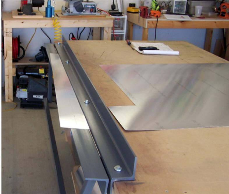
Step 1: insert part and tighten the bolts.
