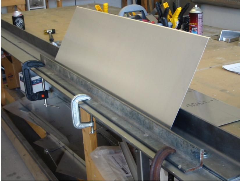
Using a piece of angle clamped to the brake to bend past 90 degrees
